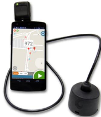
The iQuarius is a mobile, highly portable, leak detection system that utilizes the technicians Smartphone's via the Aquarius App. Using a 3G connection and GIS mapping, a leakage technician can survey areas whilst recording progress, performance and network sound samples. This can be uploaded to management dashboard and used for enhanced data analysis. As the iQuarius is simple to use it can be used by non-specialised technicians, which is excellent when urgent attention is required.
